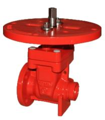
Standard: AWWA C515/BS5163 Size: DN50~DN300 Working Pressure: 200/250/300psi Body: Ductile Iron
